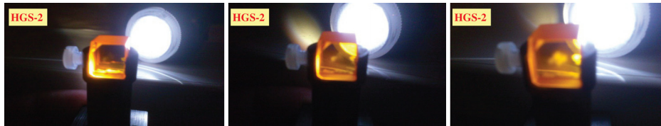
Fig. 7 Bulk damage occurring in the type-II orange-phase HGS-2 OPO element generating 6.3- \mu\text{m} idler pulses after using it for hours at >100 mJ pump energy and 10 Hz.
