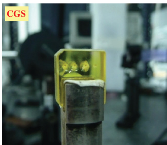
Fig. 11 Rear surface crack observed in CGS.
